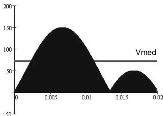
$$V_{med} = \frac{1}{T} \cdot \int_0^T |v(t)| \cdot dt$$
